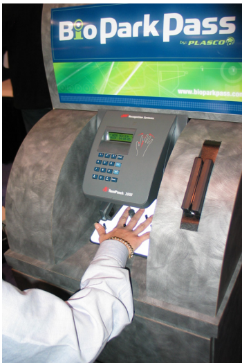
A self-serve kiosk. The pass holder is identified by the season pass' magstripe and authenticated by the hand reader.
